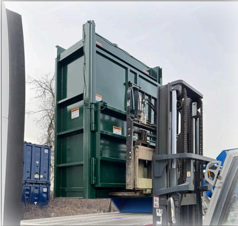
Built-in forklift pockets allow for ease of transport and installation. Baler can be easily loaded on a standard flatbed by a forklift.
