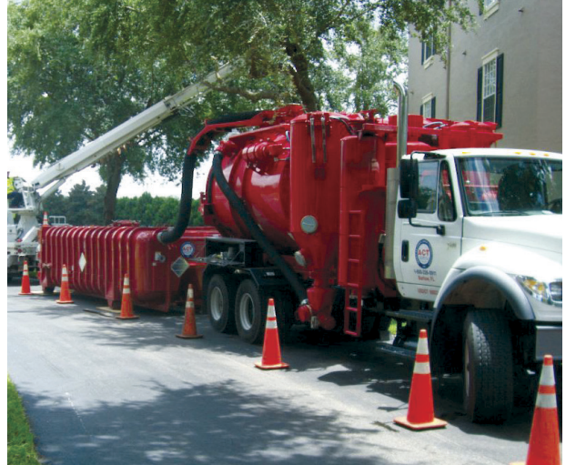
A vacuum truck bypasses its tank and pumps straight into the vacuum container, keeping the vacuum truck at the site working while vacuum containers are filled and hauled away.
